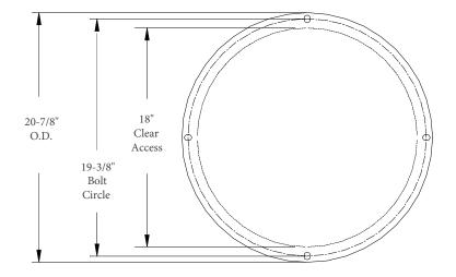
\* Stainless Steel Hardware & Gasket Tape For Gas Tight Seal Provided
